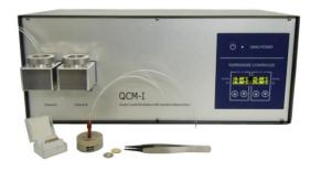
The QCM-I measuring unit is a high-sensitivity mass sensor, which measures the change in frequency of a quartz crystal resonator and as a label free biosensor it measures the "wet mass" of the adsorbed layer in processes occurring at or near the sensor surface.
